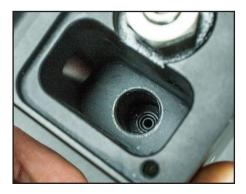
**7** Replace plastic seat and small O-ring from the pocket using a small carriage. dental pick.
