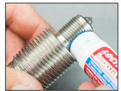
■ Apply a small amount of #248 "Blue" Loctite to the small threads.
