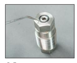
**14.** Inspect o-ring at end of the valve cartridge. If damaged, replace with large o-ring from the rebuild kit.
