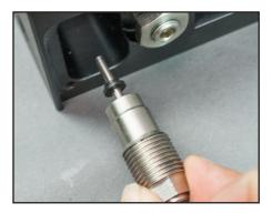
**6** Remove pin and pin carriage
