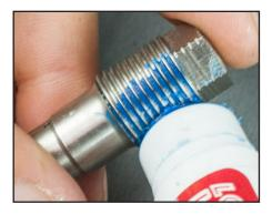
**13.** Apply a small amount of #248 "Blue" Loctite to outer threads.
