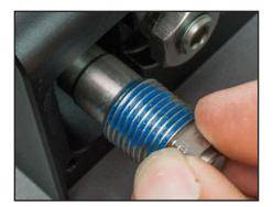
**15.** Reinstall pin carriage assembly into fill station.
