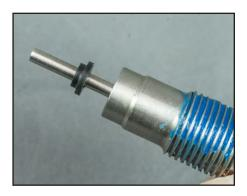
**14.** Install new seat onto pin.
