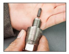
**4** Remove the plunger and spring assembly.
