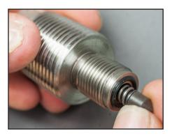
**9** Replace plunger and spring assembly into the valve cartridge.
