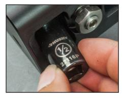
**16.** Tighten the pin carriage by hand using the 1/2" deep well socket.
