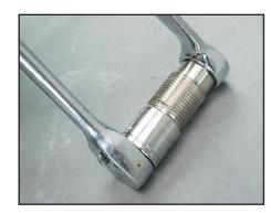
**13.** Tighten valve cartridge cap using the 7/8" wrench and the 7/8" ratchet. Tighten snugly. Torque to 45 ft/lbs.
