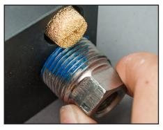
**16.** Reinstall valve cartridge
