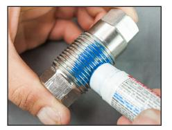
**15.** Apply a small amount of #248 "Blue" Loctite to the Large Threads.
