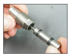
**8** Remove the pin from the pin carriage.
