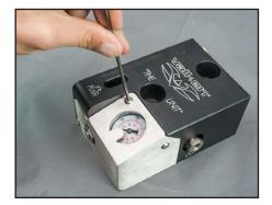
**1** Remove the gauge cover plate by removing the (4) stainless steel screws using a 1/8" allen wrench.
