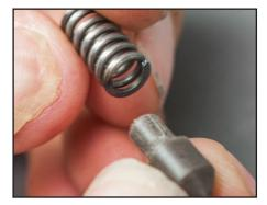
**7** Remove black plunger from spring and replace with new plunger from rebuild kit. (if needed)
