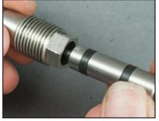
**12.** Reinstall pin into the pin carriage.
