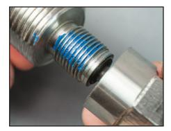
**12.** Re-install valve cartridge cap and ensure the plunger is in proper position.
