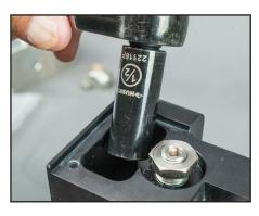
**5.** Using the 1/2" deep well socket, unscrew the 1/2" pin carriage.
