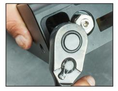
**17.** Snug pin carriage using 1/2" deep well socket and ratchet. \*Do not overtighten.
