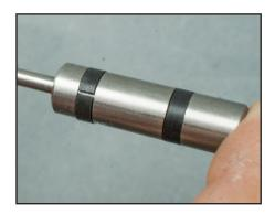
**T** Splits in split bushings should appear invisible once installed.
