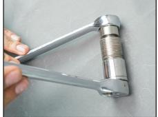
**3.** Using the 7/8" wrench and 7/8" socket, unscrew the valve cartridge cap. \*May have to heat
