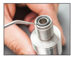
**5.** Inspect O-ring for damage.
