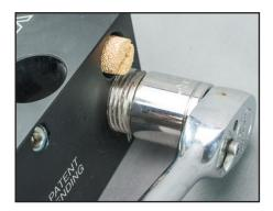
**T** • Remove valve cartridge using 7/8" ratchet. \*May have to heat
