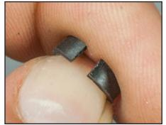
**9.** Inspect pin split bushings (they should be split). If worn, replace with new split bushings in the rebuild kit.
