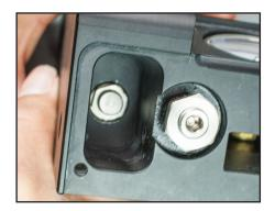
**4** Note the 1/2" Hex fastener at the bottom of the pocket.
