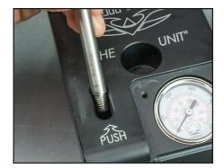
**19.** While sliding pivot into pocket, insert handle and screw into pivot.
