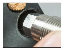
**2** Completely remove valve cartridge from filling station.
