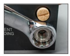
**17.** Tighten valve cartridge cap using the 7/8" wrench. Torque to 45 ft/lbs.
