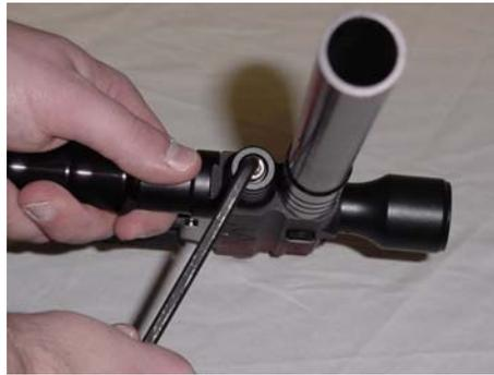
Remember that the velocity adjuster is in the front of the marker. You may be used to turning the back knob of a marker to adjust the velocity. Since our adjuster is not in the back of the marker, adjusting the knob like this may cause the back knob to loosen to the point of coming out of the marker. It could damage the spring or hammer or cause injury if there is air on the marker at the time. Remember to only adjust the velocity in the front of the marker.
