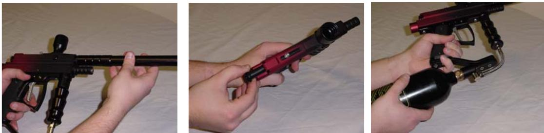
You will need to also get a loader, also known as a hopper, to carry your supply of paintballs. Because most people will want a better loader, we have chosen to not include a "cheap" loader with our marker. Attach the loader to the feed tube on the top of the marker and fill the loader with paintballs. Push the safety pin in, until ready to fire. You are now ready to fire your marker.
