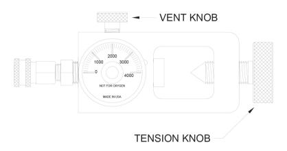
The Scuba Yoke Fill Station is designed to provide a simple, convenient way of using compressed air from a Scuba tank to refill your air system.
