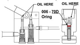
Periodically check the fill adapter and fill hose for thread integrity, cracks or other wear replace any suspect part immediately call 815-477-0007 www.ninjapaintball.com
