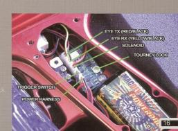
To reset the board, first enter programming mode (turn the Droid on with the trigger depressed). The interaction LED should now show blue (debounce register). Use a q-tip or similar non metallic, blunt item to depress the tourney lock button as shown. Hold the button for approximately 10 seconds until you see the indicate LED flash a rainbow of colours. The software is now reset to default settings.
