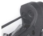
STEP 4. Remove stock ASA using 1/8" hex key. Keep stock ASA screws and mounting screw o-ring for installation of your Remote Backplate Adapter. (Fig 4)
