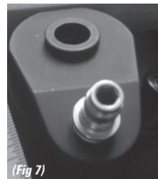
STEP 7. Apply Teflon Tape to Pro Fill Nipple Adapter and place in port. Tighten using 5/32" hex key. (Fig 7)
