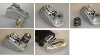
WARNING: Before applying air to marker unscrew Regulator adjustment screw to set pressure to zero as pressures may have changed during service.
