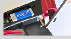
Unscrew regulator from frame (degass marker first)
