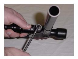
Remember that the velocity adjuster is in the front of the marker. You may be used to turning the back knob of a marker to adjust the velocity. Since our adjuster is not in the back of the marker, adjusting the knob like this may cause the back knob to loosen to the point of coming out of the marker. It could damage the spring or hammer or cause injury if there is air on the marker at the time. Remember to only adjust the velocity in the front of the marker.
