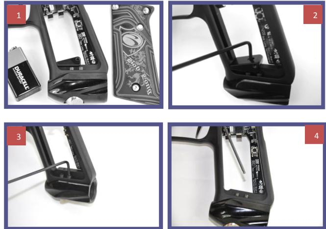
NOTE: When tightening the screws use a star pattern similar to changing a tire. If you try and tighten all of the screws completely before making sure all four are close to snug you may damage the assembly or have an unstable seal. This is the kind of damage that results in heckling by your friends and pictures with the caption of FAIL. Of course, if that happens your marker probably won't work either.
