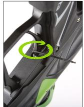
Turning the trigger adjustment screw in (clockwise) with 1.5mm Allen key will shorten the trigger pull. Moving the trigger closer to the trigger switch
