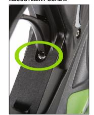
To adjust your trigger. Locate the trigger adjustment screw(S-051) on the upper portion of the trigger.
