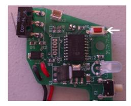
Each time the lock button is pressed while the marker is off, the LED will briefly flash green or red to indicate the status of the programming mode. If it flashes green, programming mode is allowed. By default the tournament lock is disabled, allowing the user to change settings.
