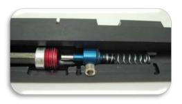
Cutaway showing Valve Wrench removing Valve Retaining Nut.
