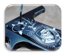
2. Loosen the Frame Screws (2 1/8<sup>th</sup> Allen Screws are submerged in the frame) that attach the frame to the marker chassis. The screws are of two different lengths – ensure you replace these properly when reassembling (shorter screw in back).
