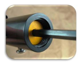
13. Insert a 1/8<sup>th</sup> Allen key into the lug and turn it until it is flush with the hammer. This allows for the removal of the hammer.
