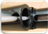
10. Note the depth of the Lug before disassembly. You want to replicate this depth upon reassembly. It will make timing the marker much easier.
