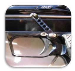
Pump the marker until you hear the sear 'click'. Holding the pump in this position adjust the undertravel screw until it touches the trigger.
