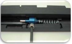
Cutaway view showing removal Valve Retaining Nut Set Screw.
