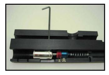
Lug adjustment shown in cutaway. Lug is at its highest point.
