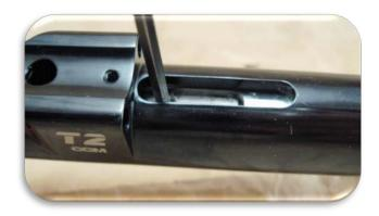
14. Remove the Valve Retaining Screw and the Valve Retaining Nut Set Screw from the bottom of the marker.
