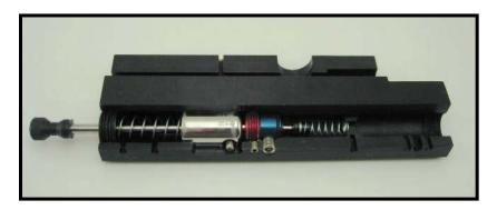
The light Valve Spring and heavier Main Spring force the valve open when not aired up.
