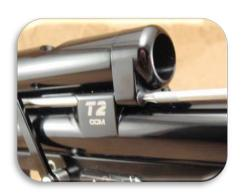
**Note:** Be very careful when replacing these screws. Use blue loc-tite and do not over tighten. Finger tight allows for smooth movement of the backblock and bolt. Over tightening of the back block screws can cause binding *once* the bolt is installed.
