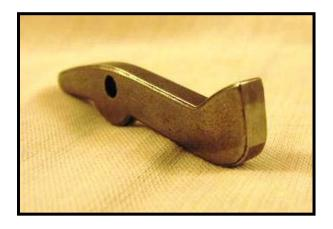
10. Remove the Trigger Shoulder Bolt and slide the trigger from the frame (shown with the top Allen key). Be sure not to over tighten the Trigger Shoulder Bolt. Over tightening can cause drag on the trigger.
