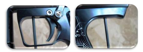
3. Now that the frame screws are loosened you can slide the AT arm off the AT lug (attached to the pump arm with Loc-tite). This will take some practice – but I find that depressing the pump arm near the lug while finessing the frame and AT arm does the trick.
