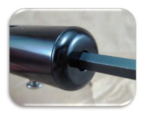
12. Remove the IVG from the marker (3/16th<sup>th</sup> Allen Key) noting its depth from flush to the rear of the body. About 3 turns are normal. The main spring will also come out at this point.
