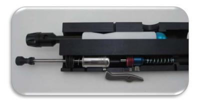
Note: This is a a cutaway of a CCM Series 5, a full block marker. The T2 works nearly the same way and seeing a cut away will help you understand what is happening inside your marker. The T2 is nearly identical to the Series 5 and 6 markers with the exception of being 'half blocked'. This is the marker cocked with a ball in the chamber.
