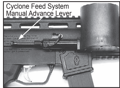
Figure 4: Manual Advance Lever for the Cyclone Feed System
