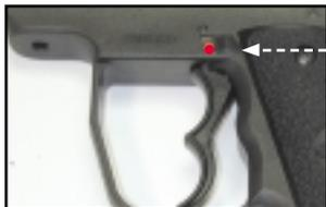
The safety is a small mechanical slide on the left side of the marker above the trigger. When the safety is “off,” a red dot is visible on the marker. The trigger can still be pulled if the safety is “on,” but the marker will not fire or de-cock.
