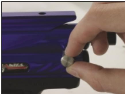
Figure 10. Remove field strip pin to begin disassembly.
