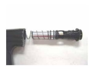
**Note:** On the top side of the bolt guide there is a small alignment hole at the rear of bolt guide. This must line up with the body alignment pin which sticks out the back of the body.
