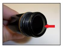
8. Apply grease to #6 Bolt O-ring and apply a light coat of grease to entire bolt.
