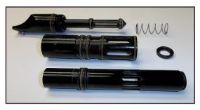
4. Unscrew the Bolt Guide from the Back Cap. Remove old grease and debris from Firing Engine.
