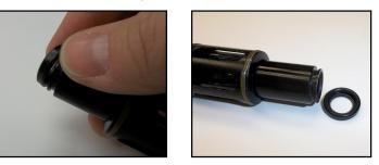
2. Unscrew the Air Guide by turning the Air Guide counter-clockwise to remove from the Back Cap. The Bolt Spring will come out with the Bolt Guide.
