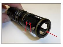
11. Apply a light coat of grease on the inner surface of the Air Guide, where the Bolt O-Rings make contact.
