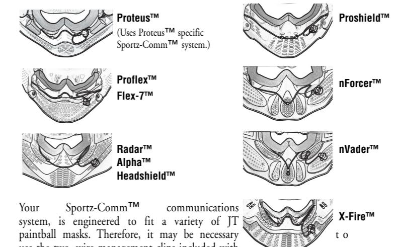
Your Sportz-Comm™ communications system, is engineered to fit a variety of JT paintball masks. Therefore, it may be necessary to use the two, wire management clips included with your system. The recommended method of wire management for your mask, is shown in one of the figures above.
