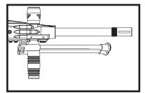
**NOTE:** If using with stock foregrip, install bipod first then the stock foregrip.
