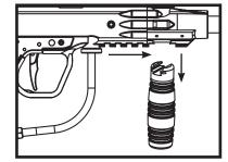
**STEP 2.** Slide Bi-Pod on to accessory rail. Make sure it is installed so that the bi-pod folds forward under the barrel. Tight both set screws with a 3/32 hex wrench.
