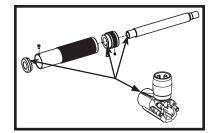
**STEP 3.** Slide the shroud over the inner barrel. Make sure the cuts in the shroud match up with the marker.
