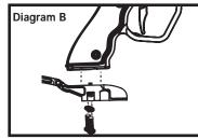
**STEP 4.** Remove field strip pin from the marker. Note: Internal are under pressure, use care.
