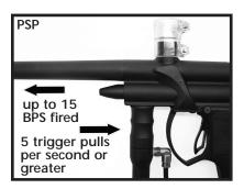
PSP Ramp (Fire Mode 2) is a tournament legal enhanced fire mode where the marker fire rate can be faster than your trigger pull rate as long as you are pulling the trigger faster than 5 pulls per second and the markers Max Rate of Fire is higher than 5 balls per second. Keep in mind that the first three trigger pulls are semi only.
