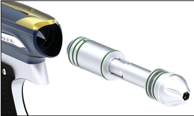
inside the supply chamber causes the bolt to start moving forward. Once the bolt has moved about half way forward, the tail of the bolt closes the input into the supply chamber. Once the Bolt reaches the forward point, the valve of the REFLEX RAIL™ Bolt is opened and air inside the supply chamber goes through the Bolt and fires the paintball.
