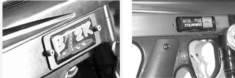
Remove the 2 screws that hold the battery cover in place. Connect the battery to the terminal and place the battery inside the frame (or tray) carefully being sure that the black and red wires to the terminal are forward and are toward the bottom. Make sure that there are no abrupt kinks and the wires are comfortably placed, do not force them into place. Replace the cover and 2 screws.
