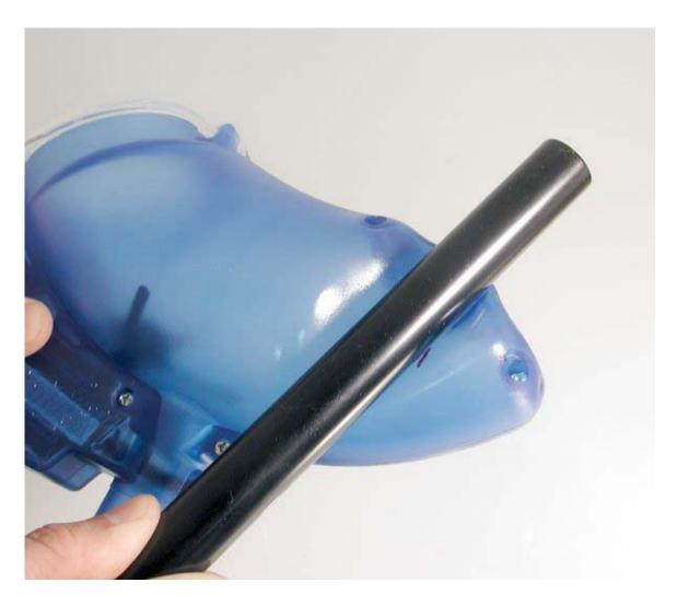
Press the barrel in and hold it for several seconds. The barrel will help cool off the plastic. Fit the hopper back on the gun to see if you need to deepen the notch anywhere. Don't be alarmed if at first you don't make a notch as deep as you planned on. Its better to err on that side! It may be helpful to go after it a little bit at a time anyway by repeating the process. This will also help give you a feel for how much heat to apply.
