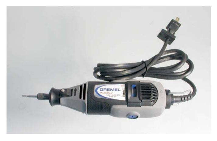
Another option would be a one inch hole saw and a drill, but keep in mind that because of the curved surface of the hopper, the holes will most likely have to be out of round. For that reason, the Dremel is superior.
