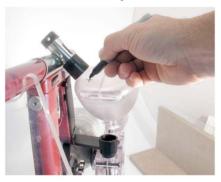
Verify the center marks by taking the power feed plug off and looking straight through the feed tube. This will insure you are in the right place.
