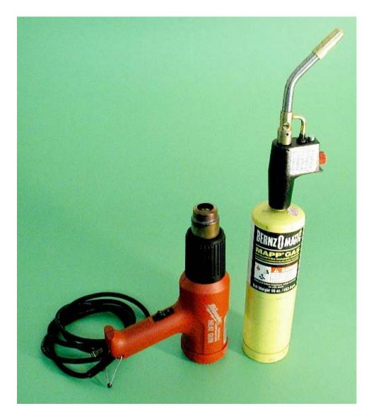
You'll need either a high wattage heat gun or propane torch and a felt tipped marker. This pictorial will show us using a heat gun but the effect is the same with the propane torch. In either case, exercise caution and safety. Do this outside or in the garage!
