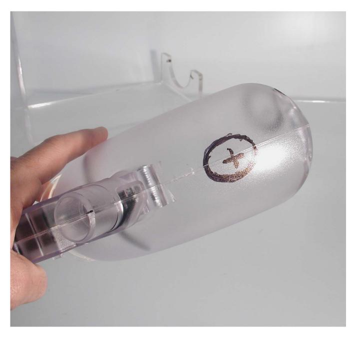
The width of the feed hose is just under one inch. Because the surface of the hopper is curved, the entrance hole will have to be elongated.
