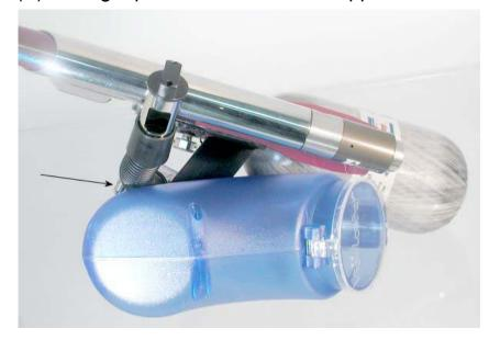
The feed hose limiting the parallel positioning of the hopper
