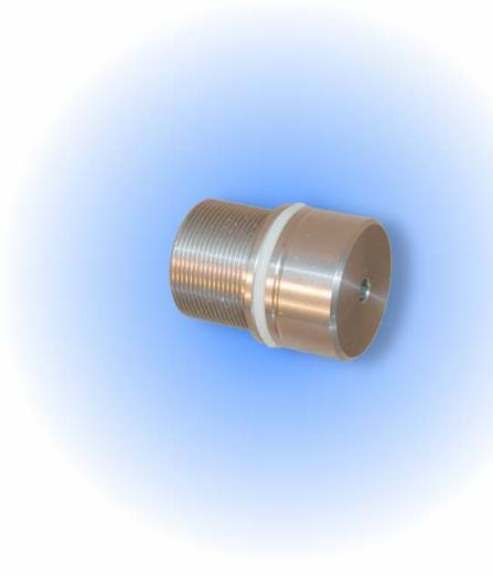
The Regulator Nut screws into the back of the valve and adjusts the velocity. Keep the threads lubricated with a good grease.
