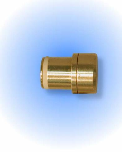
The Regulator Piston comes as an assembly that has a built-in blow off valve. Do not disassemble! Replace this part when air is venting out the back of the marker and you are shooting less than 300 FPS.
