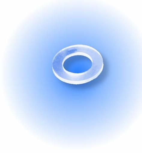
This clear urethane washer sits at the base of your power tube. When the bolt returns, it hits this to decelerate. This bumper is a little softer than the standard blue bumper for the higher firing rate of the Retro Valve. The bumper should be replaced about once a year. One Included in the Parts Kit.
