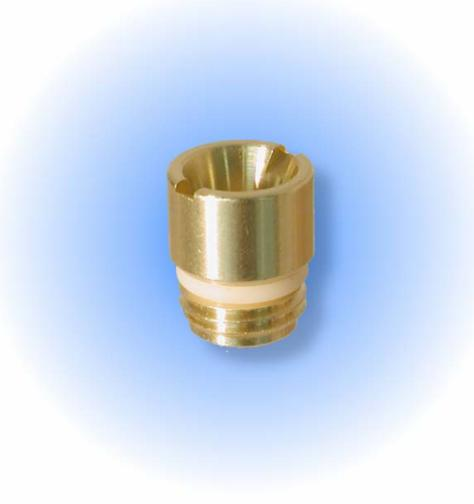
This item screws into the end of the Power Tube and is a precision part. It releases the air blast behind the ball in a controlled manner so the air hits the ball with low pressure to gently accelerate it out the barrel. Use a coin to tighten it up.
