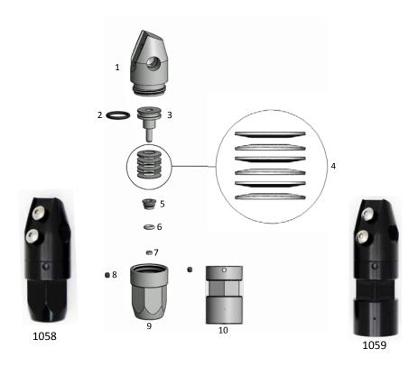
The regulator is pre-set to 750 psi with a 6 disc stack. Normally you would not change the orientation position of the discs as shown.
